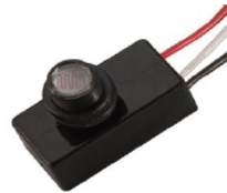
Motion Sensor Item Code: MS Part #: EHA-SENSOR-MOTION-277V Line voltage occupancy motion sensor with ambient light sensor AC110-277V mechanical relay only. External box with threaded nipple
